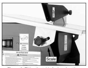
Figure 9. Tilting the table for bevel cutting.
